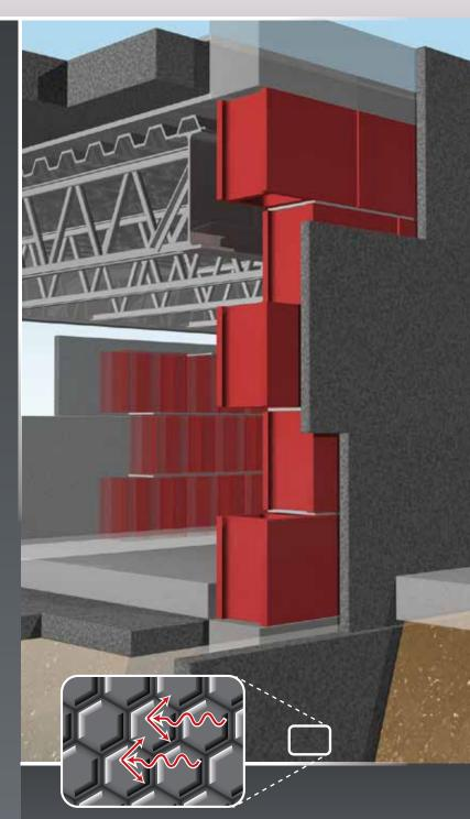
Cell-to-cell reflection of radiant energy occurs throughout the entire thickness of insulation.
