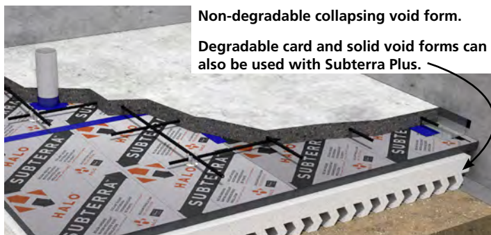
Subterra Plus as void form protection.
