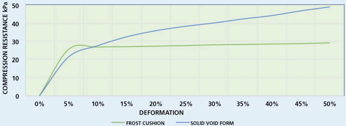
CHART 1: COMPARING FROST CUSHION TO SOLID VOID FORM UPLIFT FORCES
