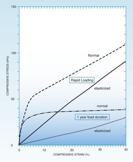
Effect of load duration on the stress-strain behavior of normal (EPS) and elasticized (EEP) expanded polystyrene block in unconfined axial compression.
